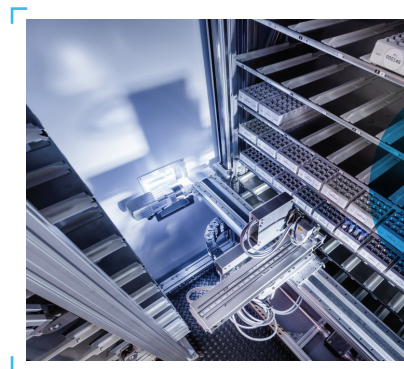
Transfer of blood samples in and out of the cold storage system
